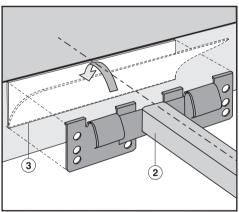
■ Position and secure the spring clamps ① and spacer bars ② using strong, double-sided adhesive tape ③.
